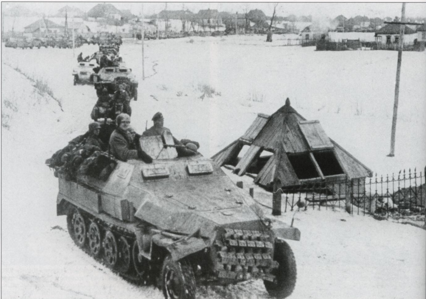
A column of Sd.Kfz. 251 armored personnel carrier belonging to the SS-Panzerkorps, which was formed in February 1943, take a detour across a snowy field near a village in the Kharkov area. Note how much equipment (particularly knapsacks) belonging to the troops is hanging on the sides of the Hanomag halftrack.
